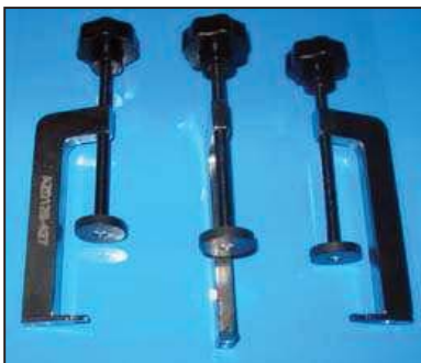
AZ0128-427- TAPPET LIFTER KIT FOR CP3 + DURAMAX Kit of 3 tappet lifters Simile 0.986.612.427 For CP3 pumps and 110 DURAMAX pumps
